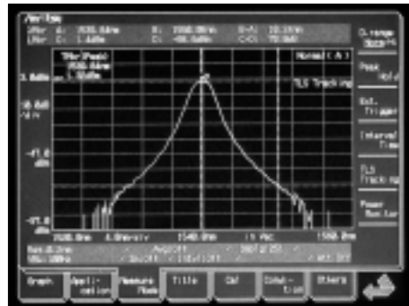
B: Wide dynamic range measurement (MS9710B display)
